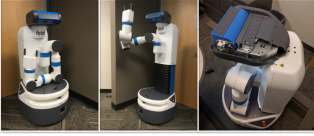
Figure 2: The Fetch in the crouched position with arm tucked (left), torso raised and arm outstretched (middle) and the rather tragic consequences of a mistaken action model (right).
