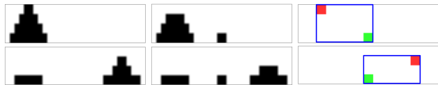
(a) Predecessor (left) and successor (middle) images of two transitions. The difference between the predecessor and successor is represented in the right images; red represents positive pixel values and green shows negative values. The blue box incorporates all pixels whose value is non-zero, i.e., whose value has changed.
