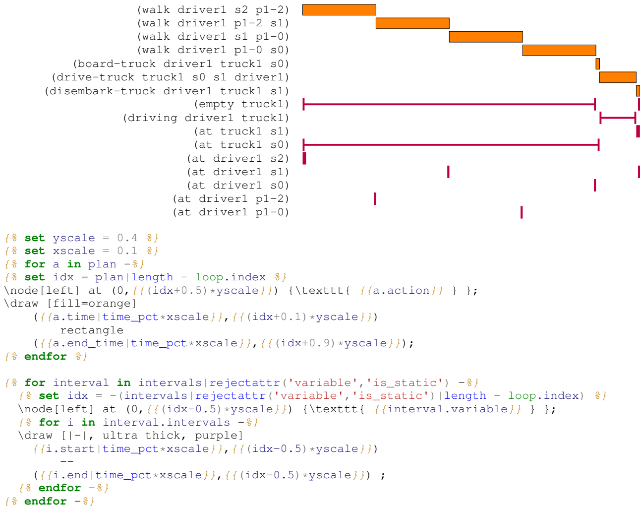
Figure 9: Plan visualisation for Driverlog Problem 1 (above) and the corresponding PDDL Template Jinja code (below) that generated the visualisation in TikZ code. This example demonstrates the use of the is_static filter which checks if a predicate is static, and the time_pct filter, which returns a time as a percentage of the overall length of the plan.
