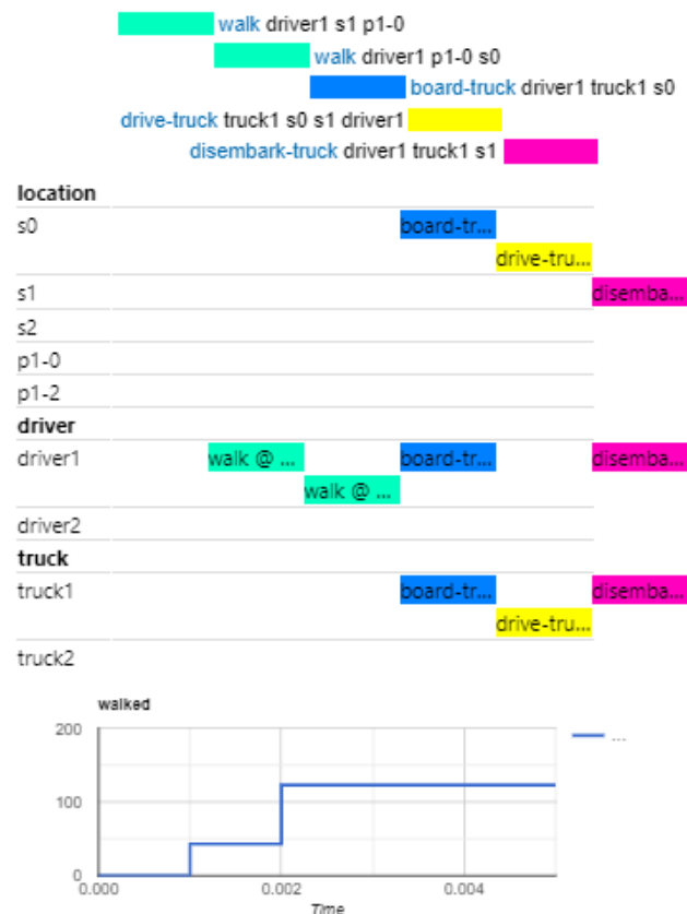
Figure 5: An example of the VS Code plan report. This report displays a Gantt Chart view of the plan, a swim-lane view for each object, and a line chart for each numeric fluent.
