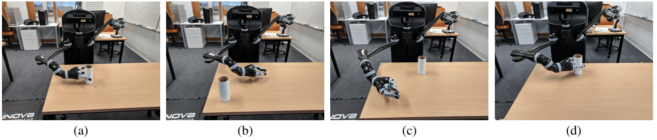
Figure 5: Snapshots of the picking task in the candy-server problem. The robot attempts to pick-up the cup (a) but the cup position is changed to the left corner of the table (b). It performs a re-localization, and attempts to pick up the cup again. But, the cup is again moved to a location close to the robot (c), resulting in the robot to attempt to re-localize the cup again. The robot then successfully picks-up the cup at its the new location (d).
