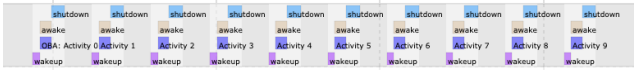
Figure 5: Sawtoothing , where each activity has its own wakeup, awake, and shutdown, occurs at low incoming SOC.
